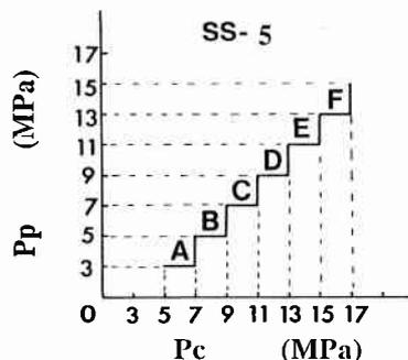
Fig.2 Schematic representation of changes in  $P_c$  and  $P_p$  of the Shirahama sandstone.
