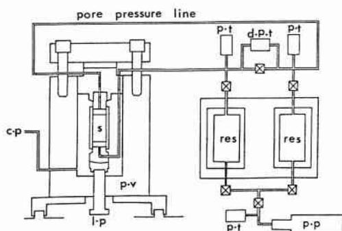
Fig.1 Schematic illustration of the pore pressure system, sample assemblage, and triaxial apparatus. s:specimen p.v:pressure vessel l.p:loading piston p.v:pressure vessel p.t:pressure transducer d.p.t differential pressure transducer res:reservoir for water p.p:pore pressure pump.
