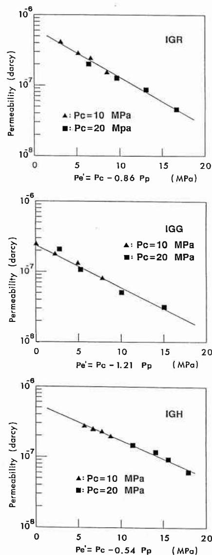
Fig.3 Permeability at modified effective pressure of the Inada granite for different preferred orientations, IGR, IGG, IGH.
