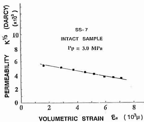
Fig.4 K versus volumetric strain for the Shirahama sandstone.
