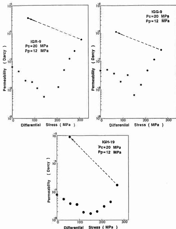
Fig.6 Permeability change as a function of axial differential stress for IGR, IGG, IGH specimens.
