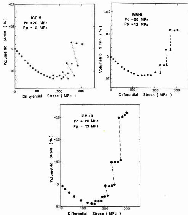
Fig.7 Axial differential stress versus volumetric strain curves for IGR, IGG, IGH specimens.
