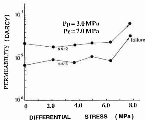
Fig.5 Permeability changes as a function of axial differential stress for the Shirahama sandstone.
